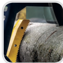
Hydraulic clamp holds log during cutting.
